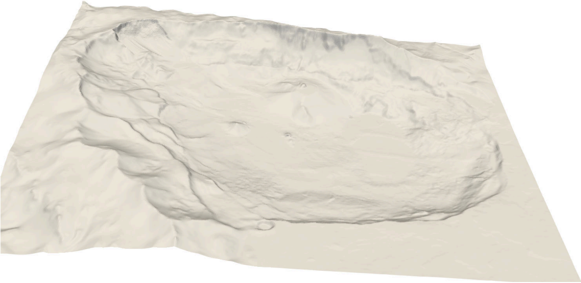
Figure 4: The terrain data without the landslide (neither initial position nor deposition) that was used to generate the mesh for the Lake Askja case.
