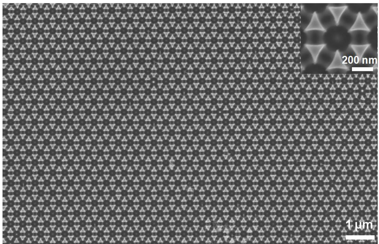
Supplementary Fig. 40 | Large-area hexagonal array of Ag nanoparticles with internally-bent triangular shape. This SEM image is obtained from the sample S3 (shown in Fig. 5a), which is characterized by the best device performance. The Ag nanoparticles possess reliable structural uniformity, which is in favor of yielding homogeneous and reproducible SERS signals over large areas.
