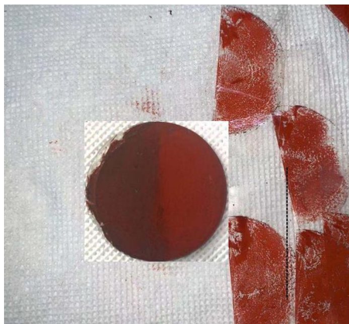
Supplementary Fig. 2. Digital photos of removing the top layer using adhesive tape.
