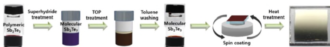
Fig. A2 Scheme of the procedures for the molecular Sb 2 Te 3 precursors and thin film fabrication (adapted from Ref. A2).
