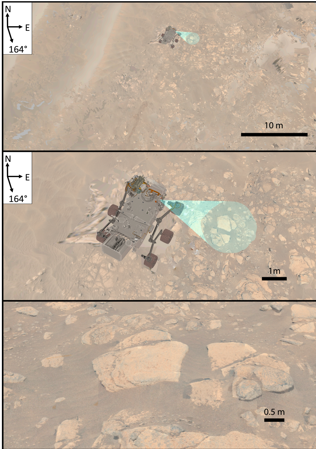
Supplementary Fig. 6 | Context images for thermal inertia measurements. (Top) A rover navigation camera (Navcam) mosaic showing the surroundings on Perseverance sol 215. (Middle) Closer view showing the approximate field of view of the Thermal Infrared Sensor (TIRS, shaded green area), used to determine the thermal inertia and albedo. (Bottom) A zoomed-in view of TIRS' field of view. The dust devil approached the rover from an azimuth of around 164° and the azimuth angle of the TIRS field of view is 102.6 degrees.
