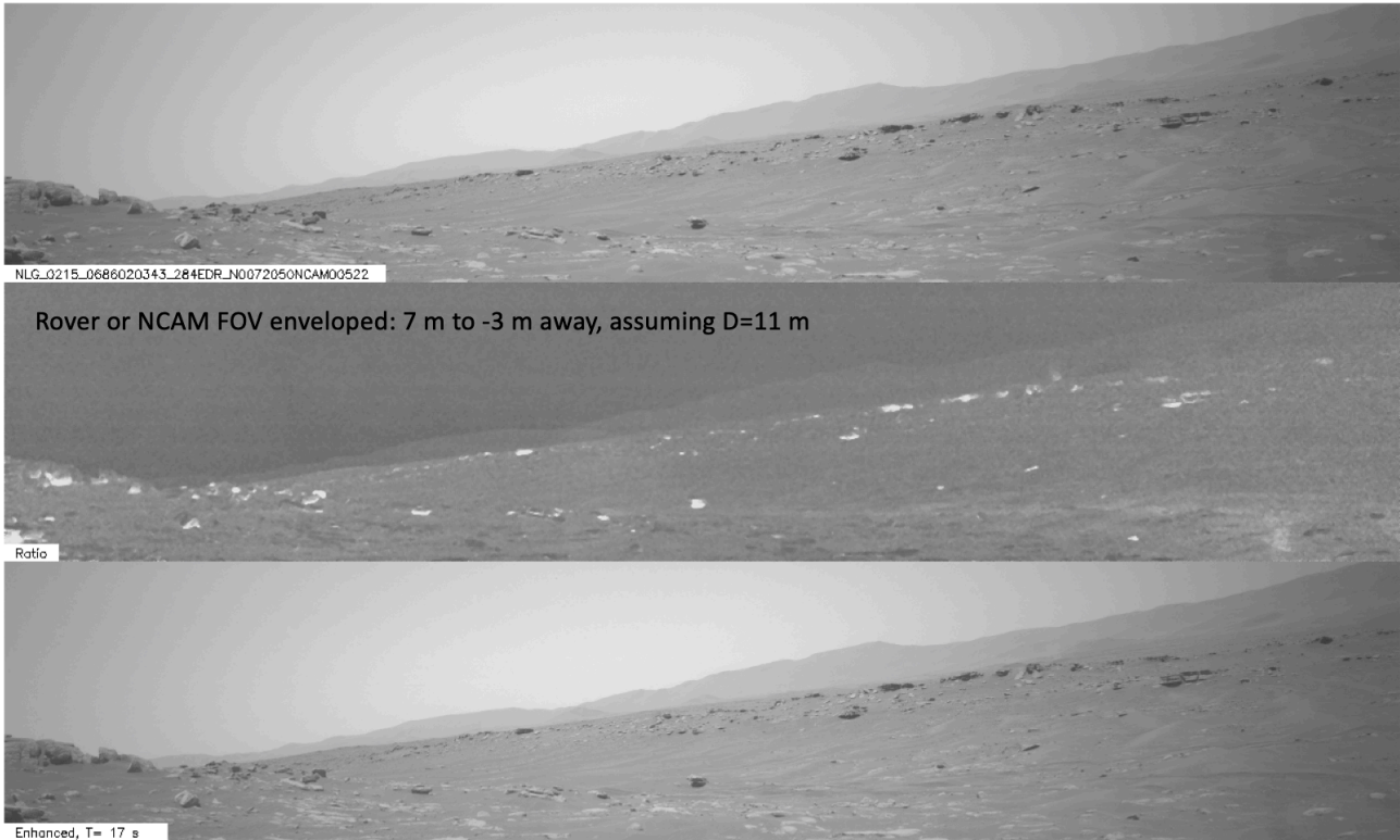
Supplementary Fig. 14 | Rover Navigation camera (Navcam) image interpretation (+4 s). (Top) The Navcam background image, (middle) the ratio of the background image and the NavCam image 4 s after the start of the SuperCam microphone recording, (bottom) the NavCam image 4 s after the start of the SuperCam microphone recording. As the rover is insight the dust devil there is no scale bar indicated the dust devil size in the middle panel.
