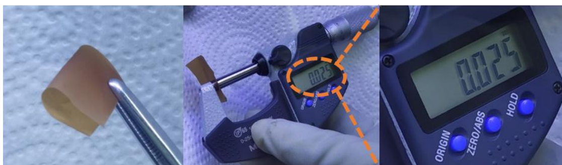
Supplementary Figure 5. HS-AlF 3 reinforced electrolyte membrane with a thinner thickness down to 25 \mu\text{m} . The thickness measurement is carried out in an Ar-filled glovebox by a high precision digital micrometer with the measurement error of 1 \mu\text{m} .
