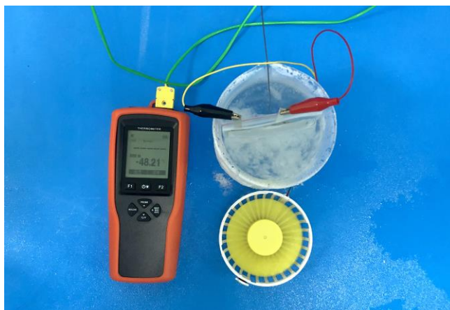
Fig. 3e. The Li||NCM811 pouch cell using the designed polymer electrolyte was powering an electric fan at about -48.2\text{ }^{\circ}\text{C} .
