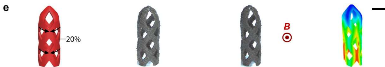
Revised Fig. 5. DIW of heterogeneous and functional thermosets. e A magnetic stent printed with 20 vol% magnetic composites. The magnetizations are in the hoop direction as highlighted by black arrows. Simulated deformed shapes agree well with experiments when the magnetic field of 50 mT is applied (scale bar=8 mm).
