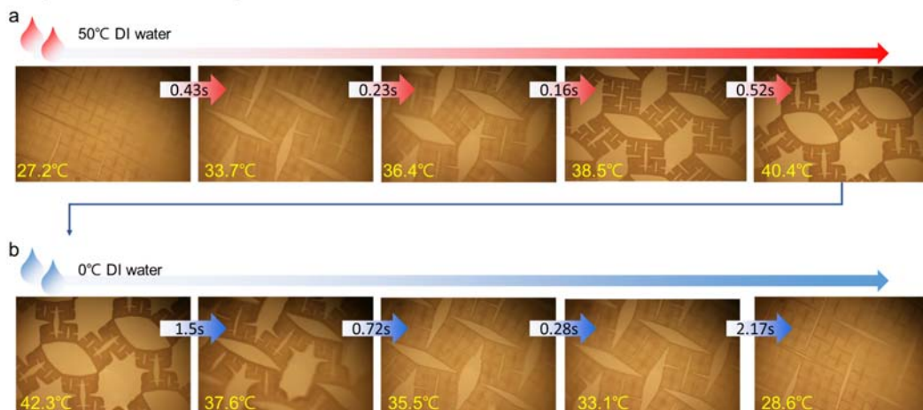
Supplementary Figure 19. Images of open and closed auxetic pattern in ATHH. a) Pouring hot water of 50°C into the ATHH in order to open the auxetic pattern and b) cold water of 0°C to close the pattern.
