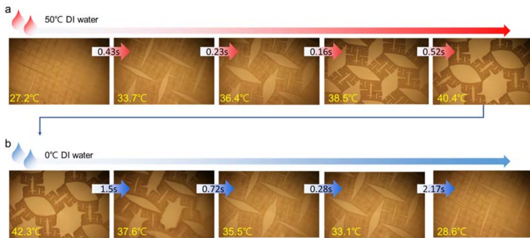
Supplementary Figure 19. Images of open and closed auxetic pattern in ATHH pouring hot and cold water. a) Pouring hot water of 50°C into the ATHH in order to open the auxetic pattern and b) cold water of 0°C to close the pattern.
