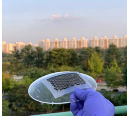
Supplementary Figure 24. A photograph of S-ATHH for large area coverage. On account of the soft lithography through the silicon etching process, the size of ATHH could be regulatable.
