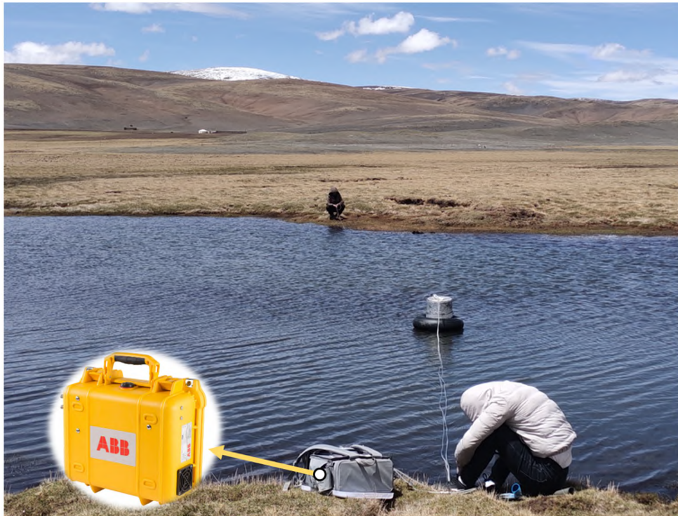
Fig. R5 Photograph of in-situ flux measurement using a near-infrared laser CH 4 /CO 2 analyzer. Photograph by Guibiao Yang.
