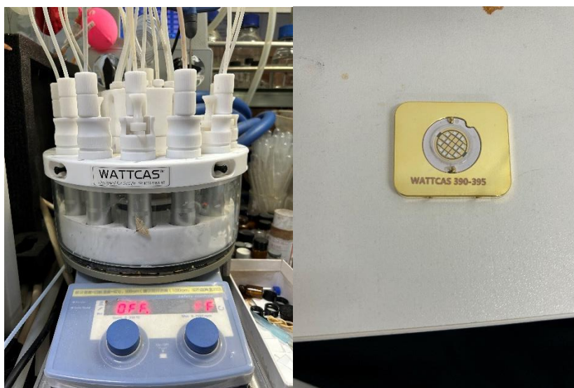
Supplementary Figure 2. Reaction setup. Left Photoreaction instrument (WPP-TEC-1020SL) from WATTCAS, Right Plank of photoreactor (390-395 nm)
