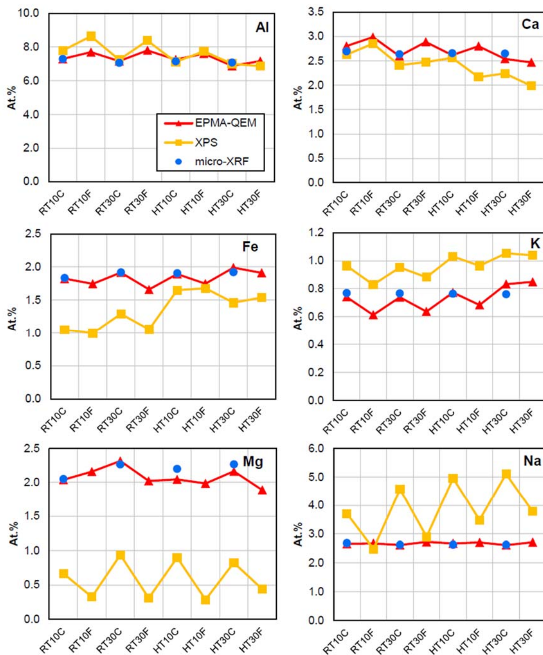
Supplementary Figure 8. Comparison of average elemental concentration from XPS (yellow squares) and micro-XRF (blue dots) measurements, and from calculations based on combined EPMA and QEMSCAN measurements (red triangles).
