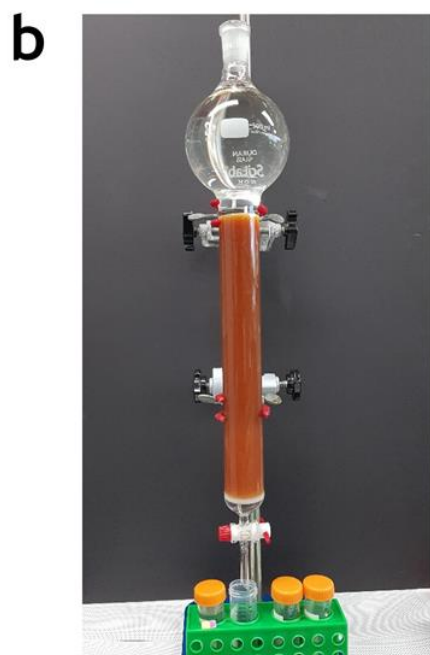
Supplementary Fig. 1. Preparing 1-ethyl-3-methylimidazolium hydroxide (EMImOH) by ion-exchange reaction. a. Scheme for ion-exchange reaction. b. Experimental setup for ion-exchange reaction. c. EMImOH product.
