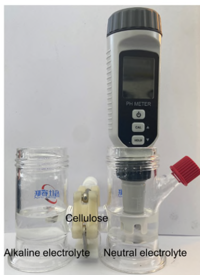
Figure R4 Digital photo of the H-cell to test barrier effect of coating.
