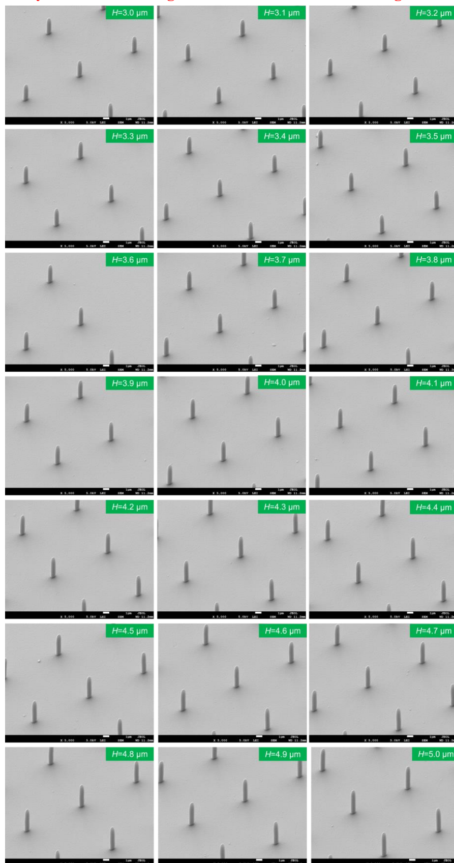
Fig. S4. SEM images of nanofins with heights varying from 3.0 μm to 5.0 μm. All nanofins have uniform transverse dimensions ( W = 400 nm and L = 800 nm).
