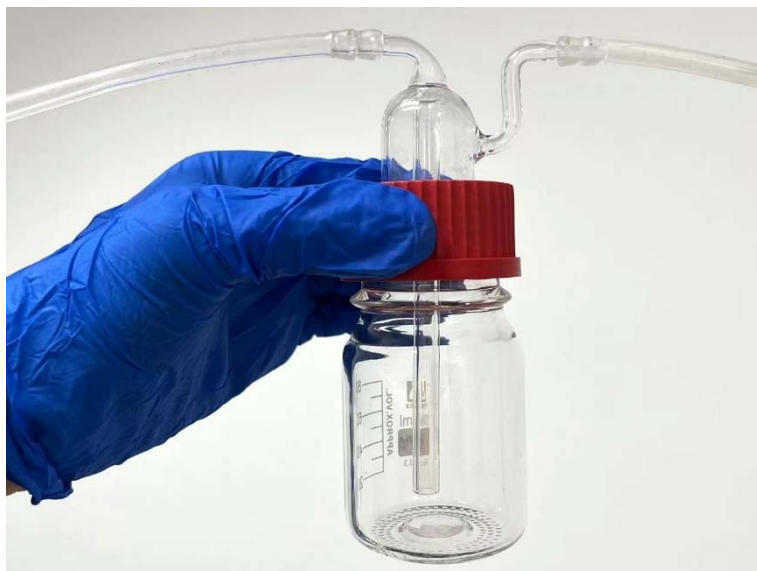
Supplementary Fig. 25 | Photograph of reactor. The seal consists of a PTFE gasket, rubber ring and silica gel grommet.
