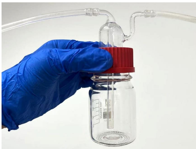
Figure R6. Schematic of reactor. The seal consists of a PTFE gasket, rubber ring and silica gel grommet.
