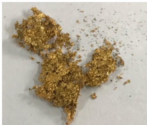
Supplementary Fig. 19. Optical photograph of the obtained gold foil from spent PyC700 in actual E-waste leachate.
