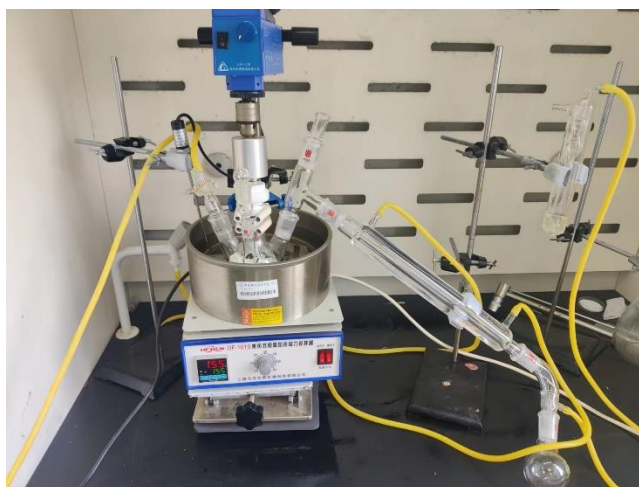
Supplementary Fig. 1. Setup used for polymerization of r -DMT to r -PET.
