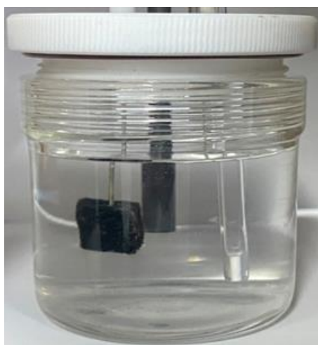
Supplementary Figure 10. Photograph of \sim 20 ppm uranium-spiked deionized water solution after 24 h of extraction using \text{Ga-N}_x\text{-C} . No solid product or other solid precipitate formed in the absence of other metal ions.
