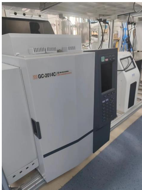
Figure S59 Chromatography measurement. Photos of the new chromatography (GC-2014C) used for calculating value of carbon balance.
