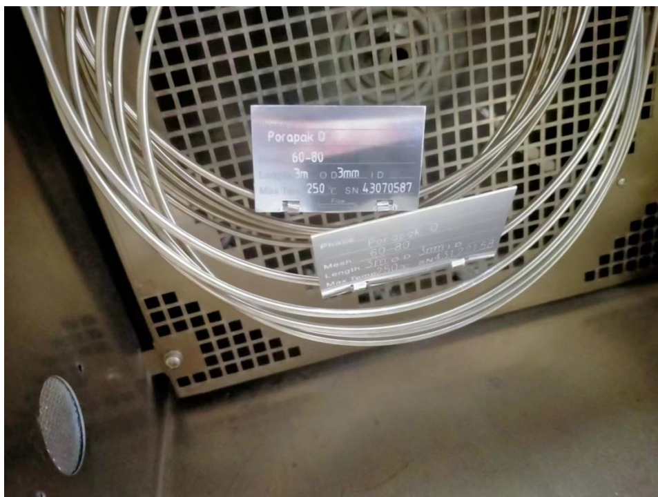
Figure S51. Photo about chromatography column. Porapak Q column used in the GC.
