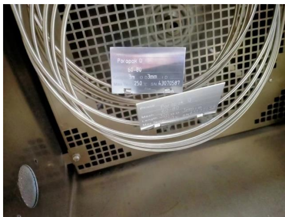
Figure S60. The picture of Porapak Q column used in the GC.
