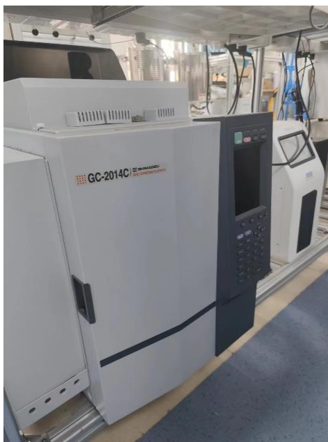
Figure S59 Photos of the new chromatography(GC-2014C) used for calculating value of carbon balance.
