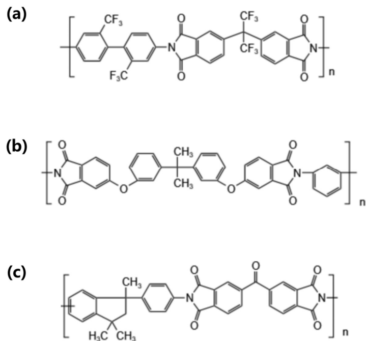
Figure S2. Chemical structures of PIs: (a) FPI, (b) PEI, and (c) SPI.
