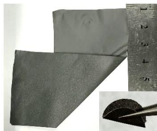
Supplementary Figure 4. Photograph of the free-standing BP electrode (named as F-BP).
