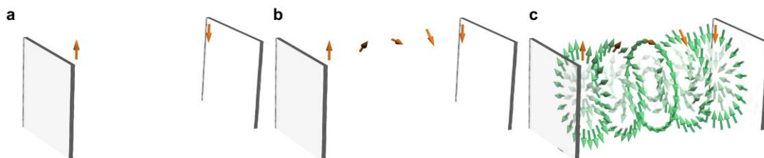
Figure R1 | Illustration of the self-assembly of a three-dimensional right-handed q -superstructure. a , Spontaneous polarization near the substrates according to the photoalignment. b , Helical structure of the spontaneous polarization with the helical axis perpendicular to the substrates. c , Three-dimensional chiral LC q -superstructure.
