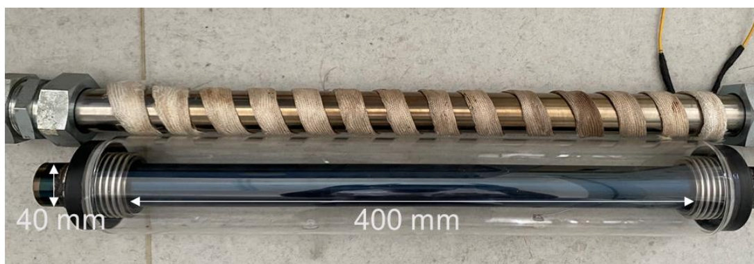
Supplementary Fig. 9. Adsorption columns for electrical heating (Top) and solar heating (Bottom).
