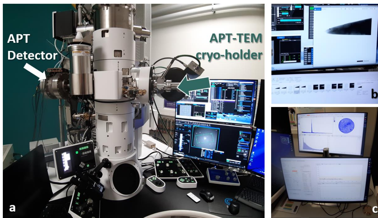
Figure S 3 : (a) JEOL F2 microscope equipped with an APT-TEM cryo-holder and APT detector both designed at GPM. (b) BF-STEM of a specimen and (c) sequence of acquisition of an Al-alloy.
