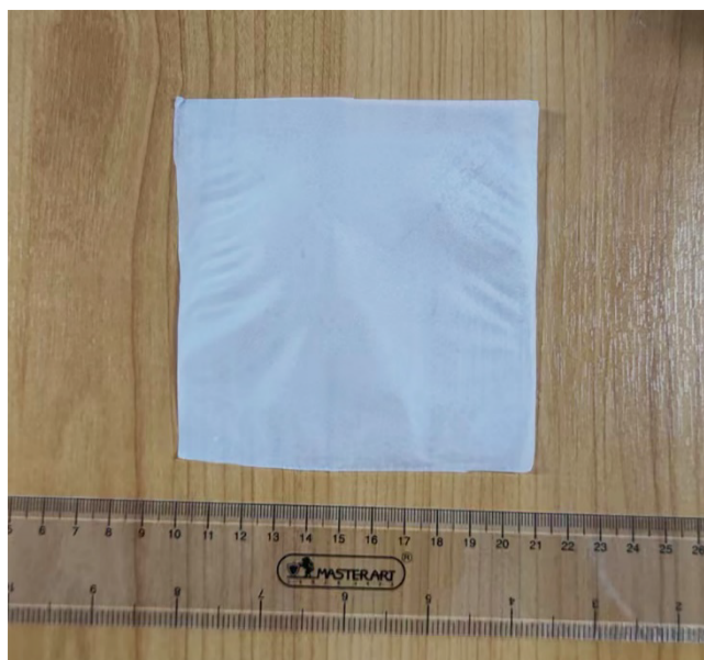
Supplementary Fig. S3 The digital photo of the polymer film after dried the PAAS-LMS-CNF solution.
