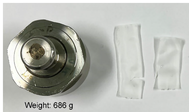
Supplementary Fig. S6 The digital photograph of PLCZ without \text{ZnSO}_4 immersion after strain-stress test. The weight for strain-stress test is 686 g.
