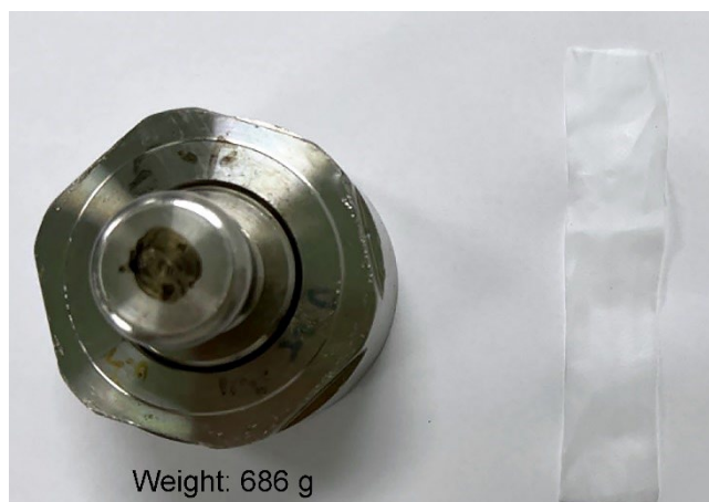
Supplementary Fig. S7 The digital photograph of PLCZ with \text{ZnSO}_4 immersion after strain-stress test. The weight for strain-stress test is 686 g.
