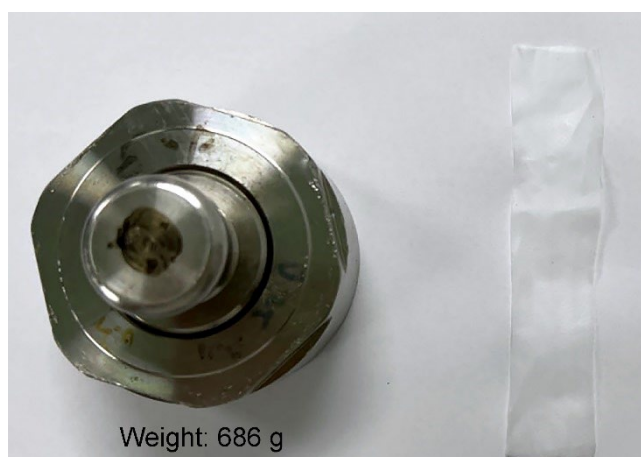
Fig. R21 The digital photograph of PLCZ with \text{ZnSO}_4 immersion after strain-stress test. The weight for strain-stress test is 686 g.
