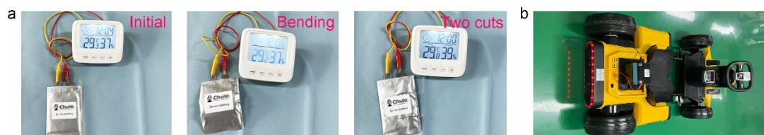
Fig. R43 The digital photographs of pouch cell (a) supporting electronic device under initial state, bending and cutting and (b) running a toy car.
