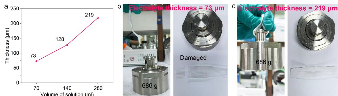
Fig. R7 (a) The thickness of the polymer electrolytes. The strain-stress tests of when the electrolyte thickness is (b) 73 and (c) 219 \mu\text{m} . After strain-stress test, the electrolyte with the thickness of 73 \mu\text{m} is damaged, but when with 219 \mu\text{m} , it keeps unwounded,
