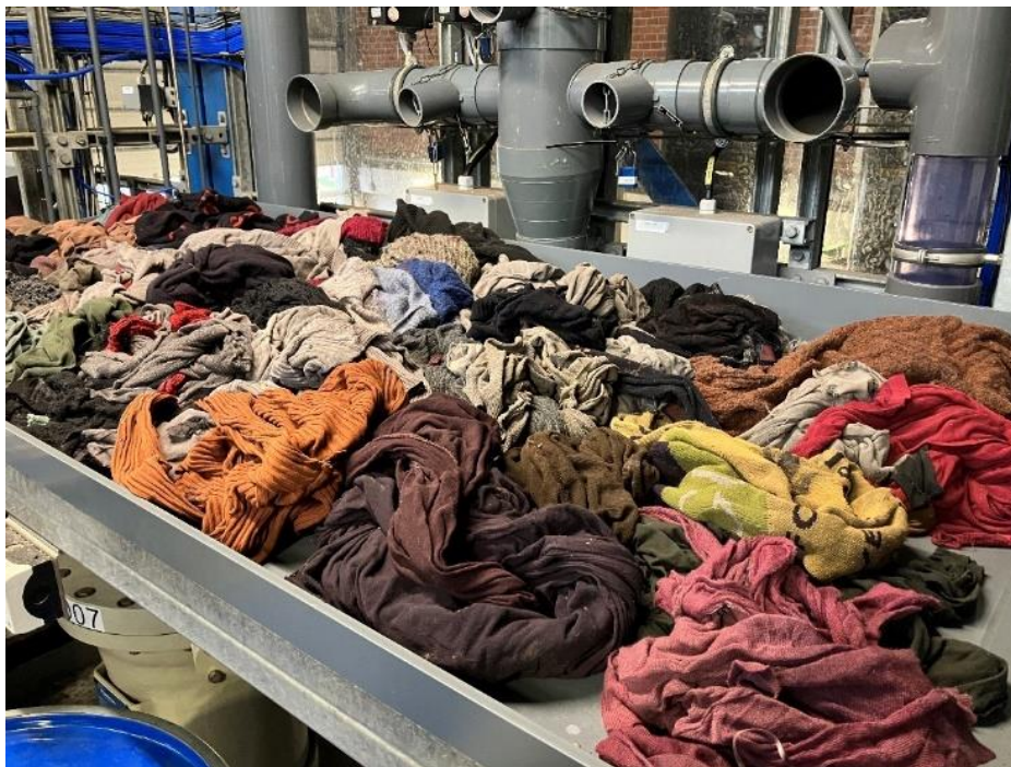
Figure S13: Polyester residue of postconsumer polycotton waste textiles after hydrolysis with 43 wt% aq. HCl in the DAWN pilot plant (run 3).
