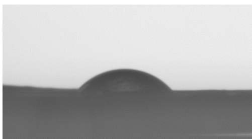
Fig. R2. The contact angle between the hydrophilic Daramic membrane and water.
