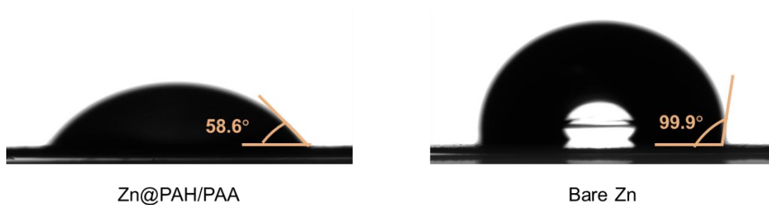
Figure S8. Contact angle test of 2\text{M ZnSO}_4 on Zn@PAH/PAA and Bare Zn.
