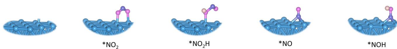
Supplementary Figure 52 | Adsorption model of reaction intermediates on Cu MPs surface.
