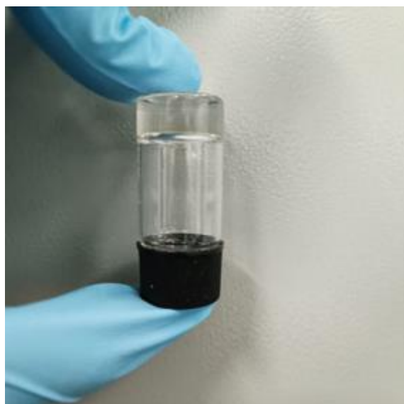
Supplementary Figure 2. Optical photograph of WSGPE electrolyte. WSGPE is a homogeneous transparent gel.
