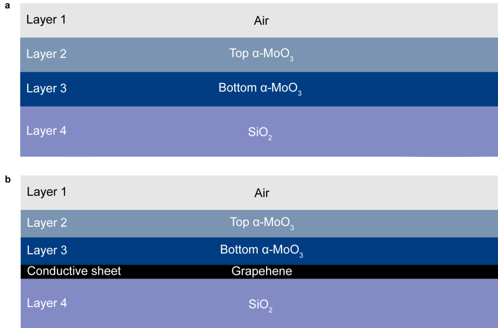
Supplementary Figure 5. Illustration of the structures used in transfer matrix method. a Layered structure of the twisted bilayer \alpha\text{-MoO}_3 . From top to bottom, it represent air, top \alpha\text{-MoO}_3 layer, bottom \alpha\text{-MoO}_3 layer, and \text{SiO}_2 , respectively. b Layered structure of the twisted bilayer \alpha\text{-MoO}_3 /graphene. From top to bottom, it represent air, top \alpha\text{-MoO}_3 layer, bottom \alpha\text{-MoO}_3 layer, graphene, and \text{SiO}_2 , respectively.
