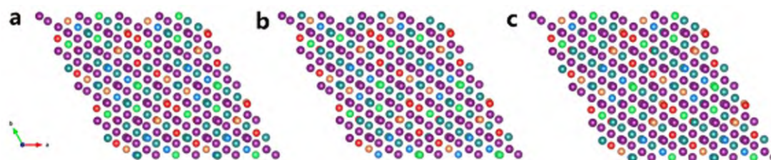
Figure S49. (a-c) A series of defect PD-PFCNZ-HEI (111) surface models were constructed by replacing the three different Zn sites on the surface with Pt. The energies of these three models are: -382.18 eV, -382.02 eV, and -377.76 eV, respectively. Therefore, Figure S49a was selected as the most stable Pd-PFCNZ-HEI (111) model with Zn sites substituted by Pt antisite defects.
