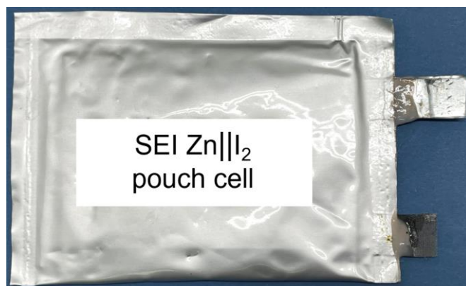
Supplementary Fig. 64 | Digital image of the assembled aqueous SEI Zn||I 2 pouch cell.
