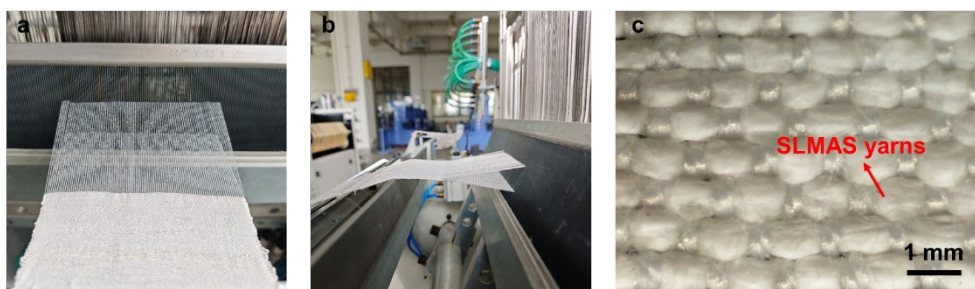
Supplementary Figure 5. a-b Photographs showing the weaving process of the conductive fabric, which is woven from commercial yarns and SLMAS yarns. c Photomicrograph of a conductive fabric woven from a mixture of commercial yarns and SLMAS yarns.
