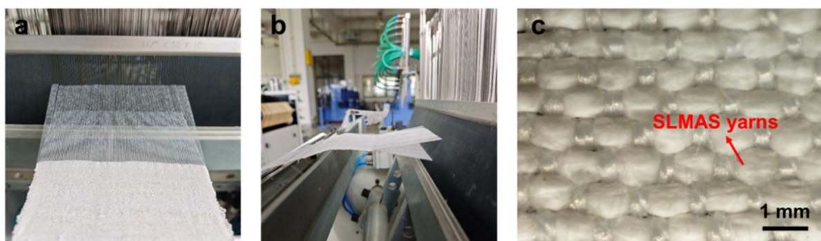
Fig. R1-13. a-b Photographs showing the weaving process of the conductive fabric, which is woven from commercial yarns and SLMAS yarns. c Photomicrograph of a conductive fabric woven from a mixture of commercial yarns and SLMAS yarns.
