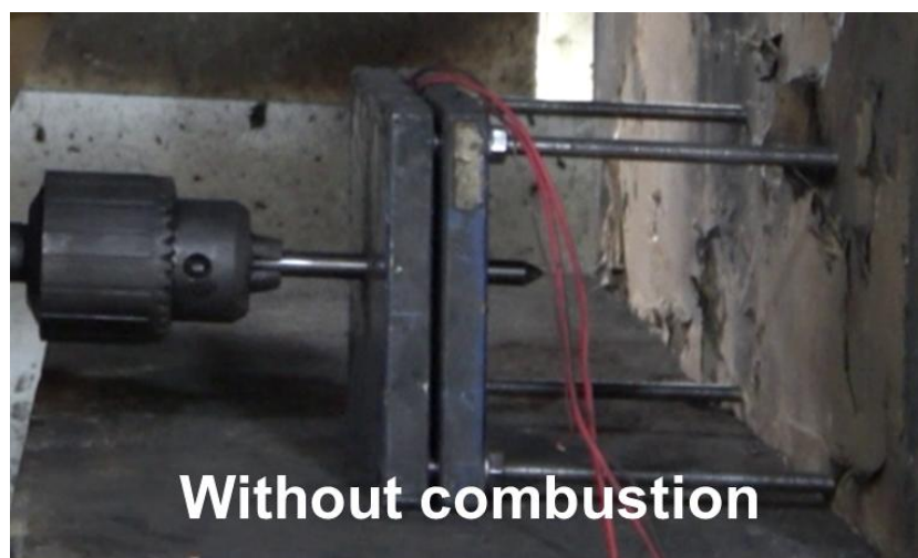
Figure S36. The nail penetration test of the 1.0-Ah Li|IWSWN-SPE|NCM811 pouch cell.
