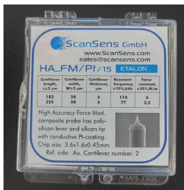
Package of the tip used in our KPFM test.
