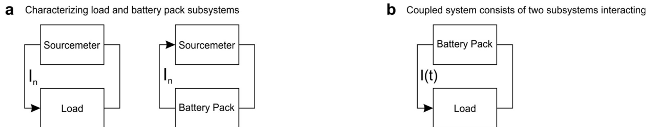
Supplementary Figure 11 | a ) Characterization of two subsystems using step function I_n b ) Direct interaction of two subsystems over time resulting in dose current
