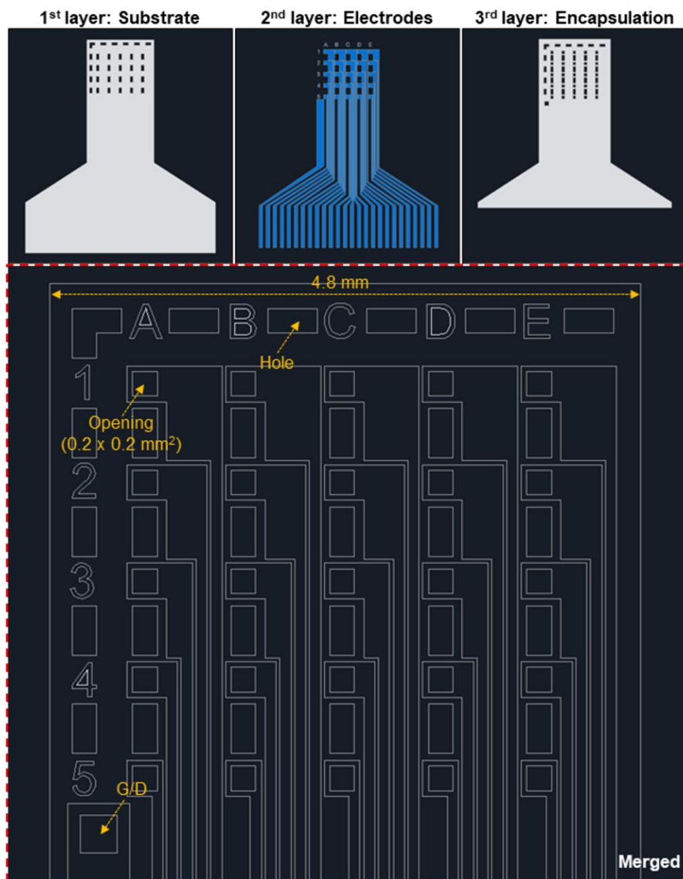
Figure S20. Device architecture of a soft, stretchable, transient epidural electronics (active area, 4.8 x 4.8 mm 2 ) featuring a 5 x 5 passive neural electrode array.
