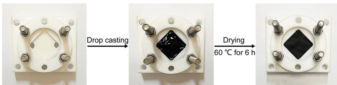
Supplementary Fig. 3 | Membrane preparation. Schematic illustration and digital images of the membranes prepared with the slurry.
