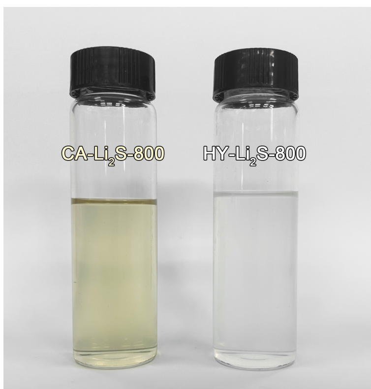
Supplementary Figure 4 | Digital picture of HY-Li 2 S-800 and CA-Li 2 S-800 after dissolved in absolute alcohol. The CA-Li 2 S-800 synthesized from Li 2 CO 3 exhibits a pale yellow color in ethanol, while the HY-Li 2 S-800 synthesized from LiOH appears greyish white indicating that these two Li 2 S products differ in properties, confirming that Li 2 CO 3 cannot be used as a substitute for LiOH in the production of Li 2 S.
