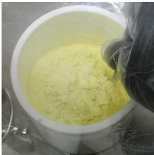
Supplementary Figure 9 | The ball-milled LPSC 1.5 -SmetaLi 2 S precursors. 34.47 g as-synthesized Li 2 S, 23.85 g LiCl and 41.68 g P 2 S 5 were mixed into 1 L ZrO 2 pot with 80 ZrO 2 balls of 10 mm diameter and 180 ZrO 2 balls of 5 mm diameter. The LPSC 1.5 -SmetaLi 2 S yellow precursors can be obtained after 8 h ball-milling with a rotational speed of 400 rpm.
