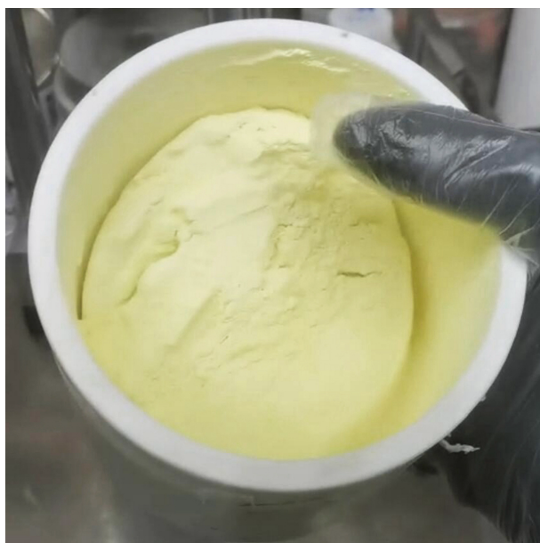
Supplementary Figure 6 | The ball-milled LGPS-SmetaLi 2 S precursors. 39.02 g as-synthesized Li 2 S, 23.23 g GeS 2 and 37.75 g P 2 S 5 are mixed into 1 L ZrO 2 pot with 80 ZrO 2 balls of 10 mm diameter and 180 ZrO 2 balls of 5 mm diameter. The LGPS-SmetaLi 2 S yellow precursors can be obtained after 8 h ball-milling with a rotational speed of 400 rpm.
