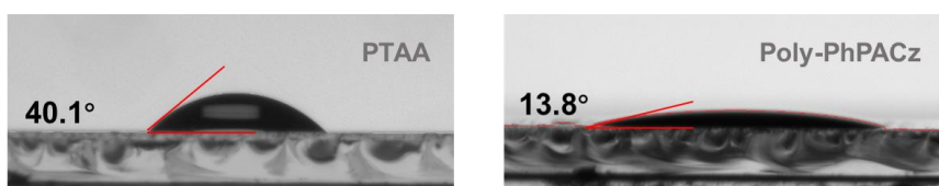
Supplementary Fig. 8. Contact angles of the perovskite ink on the ITO substrates coated with PTAA and Poly-PhPACz.
