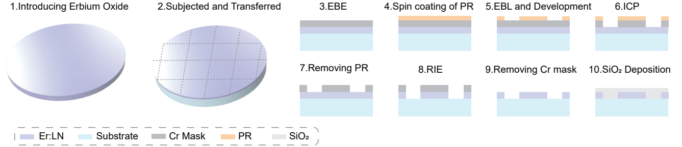
Fig. S2. The Er:TFLN PIC fabrication process consisting of the ICP-RIE process
