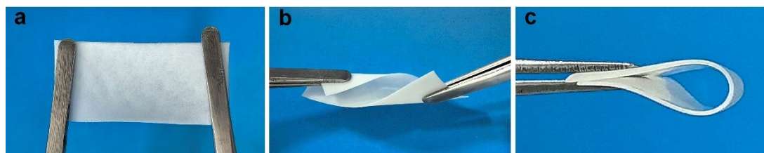
Fig. R26. Photographs of the self-supporting IHCE membrane in its original (a), wrapped (b), and folded states (c).
