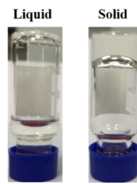
Figure S8. The hydrogelation ability of Matrigel before and after being heated at 37 °C for 10 min.
