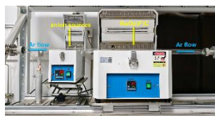
Supplementary Fig. 80. Schematic diagram of the heat treatment synthesis process for M–RuO 2 /(F)C (M = N, S, P, Se, Cl and Br) using tube furnace.
